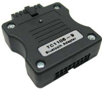
Plug-In Bluetooth Module
